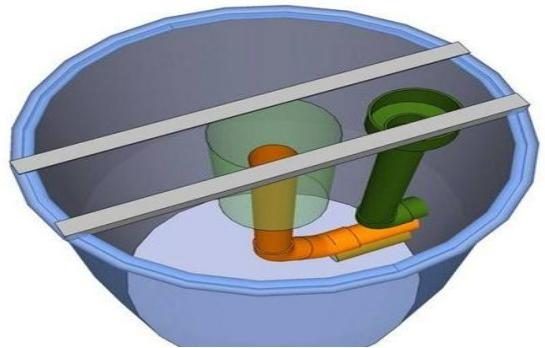
**Figure 6:** Solidworks Drawing: Simulation of a settler
