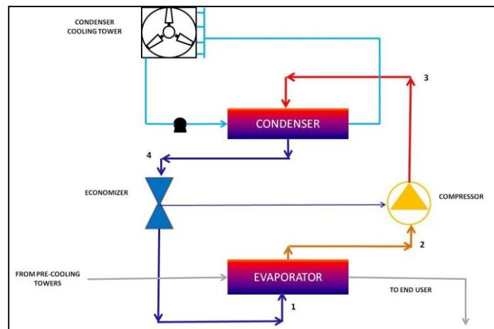
**Figure 3:** Refrigeration Cycle
