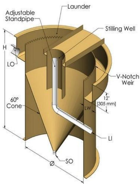
**Figure 5:** Solidworks Drawing: Cross section of a settler
