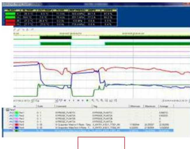
Figure 5: SCADA System showing the system fluctuation during heat exchanging process
