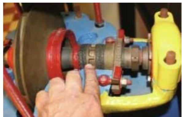
**Figure 1.** Centrifugal pump seal under investigation.
