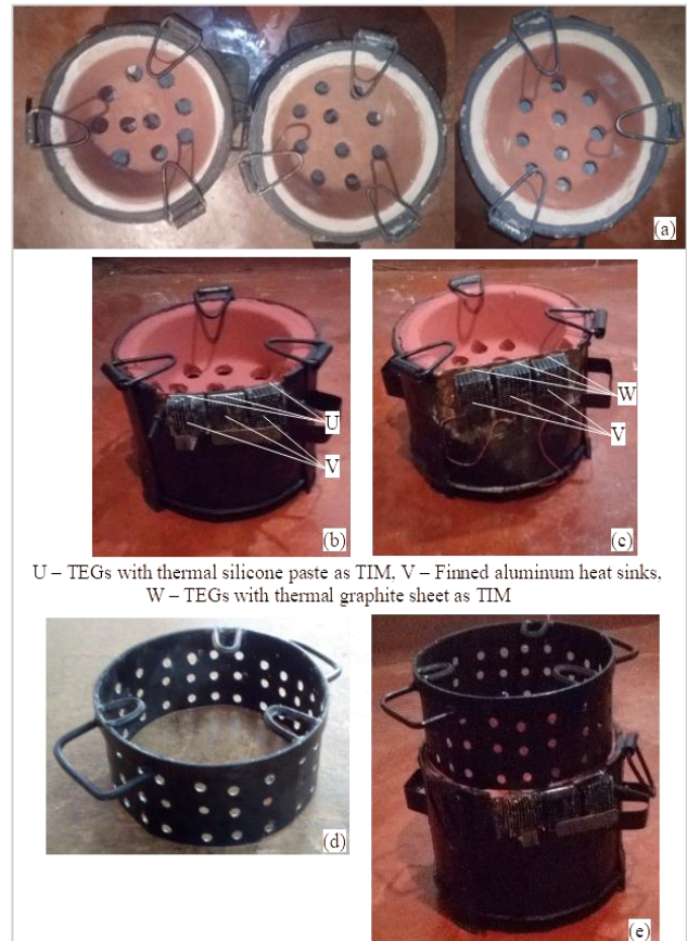
Figure 5: (a) KCJ cookstoves before modifications, (b) cookstove with thermal silicone paste as TIM, (c) cookstove with re-used thermal graphite sheet as TIM, (d) Perforated rolled steel sheet, and (e) Modified KCJ and perforated rolled metal sheet for facilitating space heating atop
