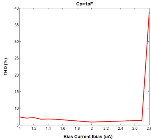
**Figure 9:** Total Harmonic distortion vs  $I_{bias}$  ( $C_p=1pF$ )
