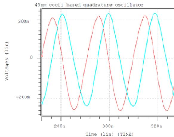
**Figure 4:** Expanded view of the output signal at node (3) and (4) of the fig.3
