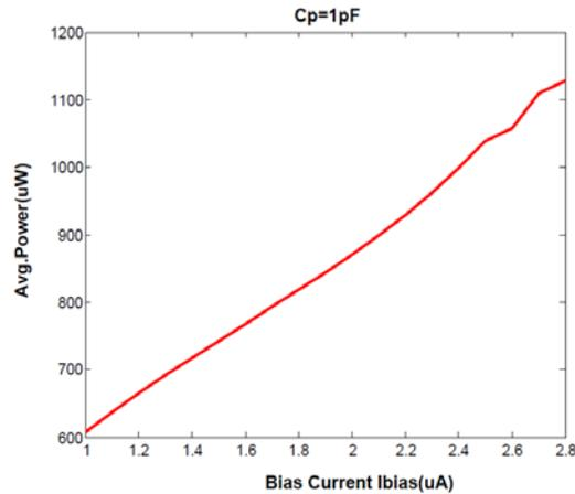
**Figure 7(a):** Avg Power vs I<sub>bias</sub>(C<sub>p</sub>=1pF).
