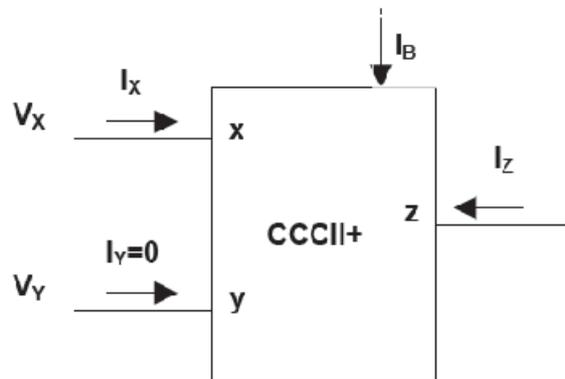
**Figure 1:** Block Diagram representation of the 2<sup>nd</sup> generation CCCII+.
