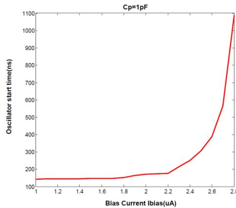
**Figure 6(a):** Oscillator start time vs  $I_{bias}$  ( $C_p=1\text{pF}$  constt.).
