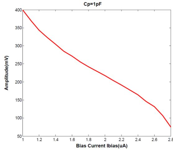
**Figure 8(a):** Amplitude vs I<sub>bias</sub>(C<sub>p</sub>=1pF)
