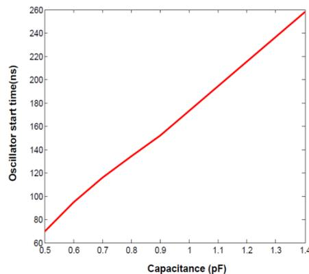
**Figure 6(b):** Oscillator start time vs Capacitance ( $I_{bias}=2\text{uA}$  constt)
