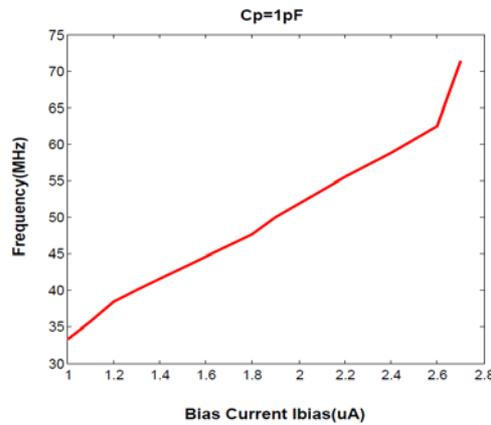
**Figure 5:** (a) Frequency vs I<sub>bias</sub> (C<sub>p</sub>=1pF constt.)
