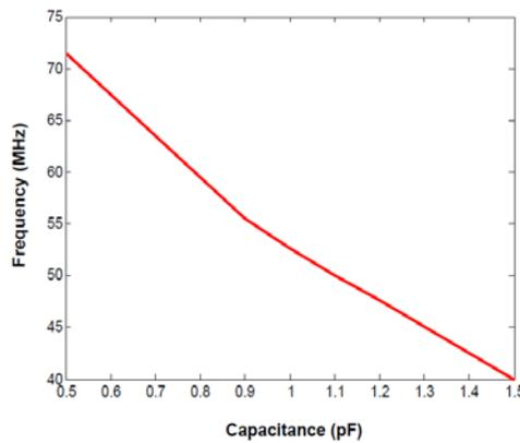
**Figure 5:** (b) Frequency vs Capacitance (I<sub>bias</sub>=2 $\mu A$  constt.)
