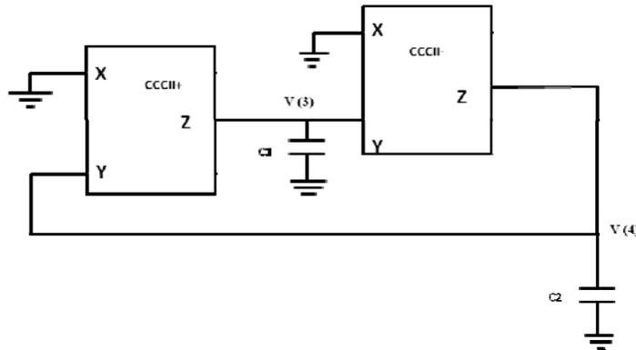
**Figure 2:** Block diagram of Quadrature Oscillator using CCCII±
