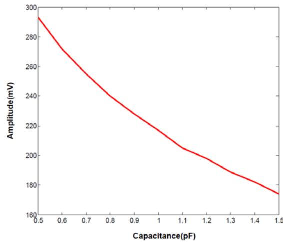
**Figure 8(b):** Amplitude vs Capacitance(I<sub>bias</sub>=2uA)
