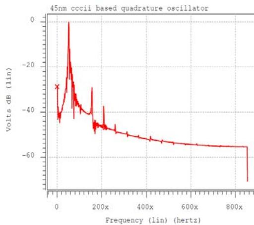
**Figure 10:** Fourier analysis of the signal at node (3) of fig (3)
