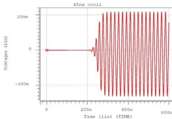
**Figure 3:** Output of the proposed oscillator (node 3).  $I_B=2\mu A$  ,  $C=1pF$ , oscillation startup time 170ns
