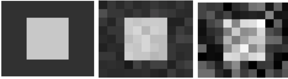
Figure 2.7: The effect of different Gaussian noise levels: (a) no noise; (b) added noise \sigma = 10 ; (c) added noise \sigma = 40 .
