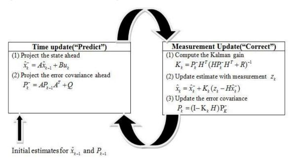
Fig. 4 A complete picture of the operation of the Kalman filter
