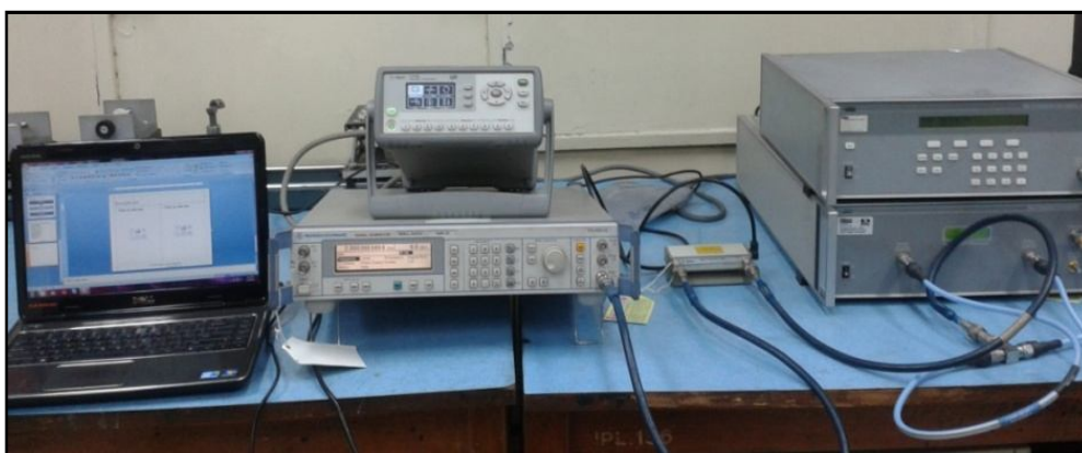
Figure 1: Measurement Setup. The hardware consists of a PC, Signal Generator, Attenuator Driver and a precision receiver, VM-7.
