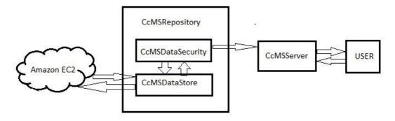
Figure 1: Architecture of CcMS.
