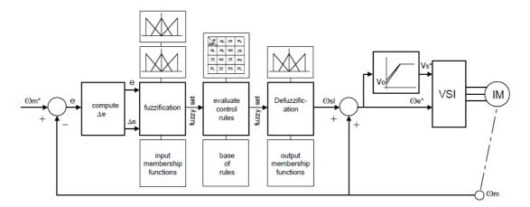
Fig1: basic block diagram of speed control of induction motor using FLC
