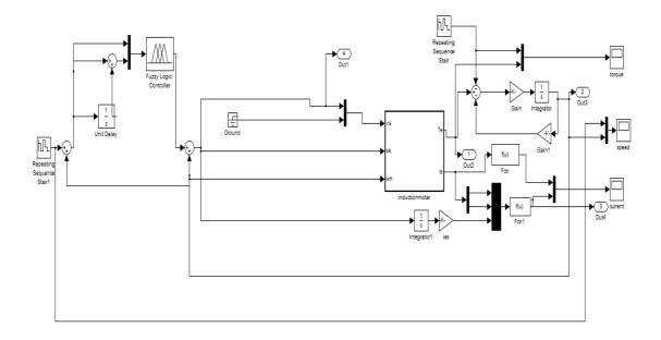
Fig.5.Circuit diagram of speed control of induction motor using FLC in Simulink
