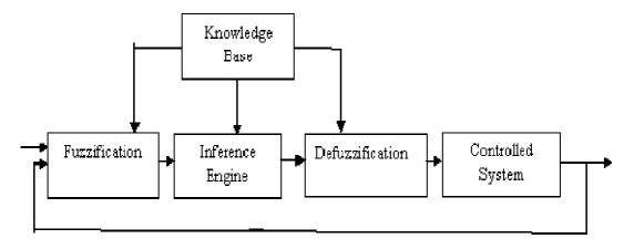
Fig.2. Basic configuration of fuzzy logic controller
