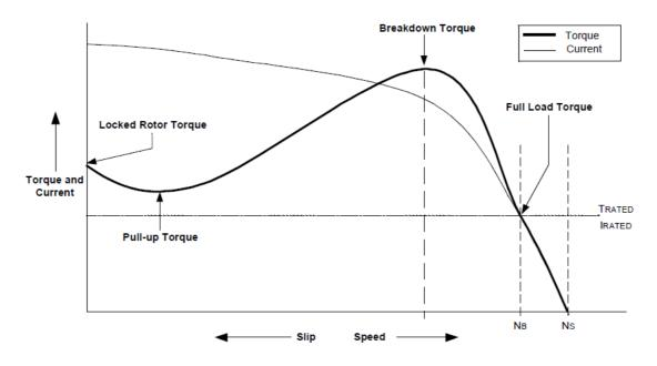
Fig.3. Torque-speed characteristics of induction motor [7]
