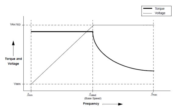
Fig.4. torque-speed characteristics of induction motor VF control [7]
