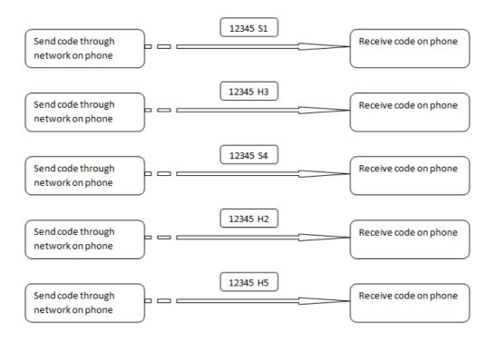
In this code shown in figure first five digit random code has been put by receiver and next two words is showning which technique is used in this 'S1' means symmetric key 1, 'S4' means symmetric key 4, 'h2' means hash function 2, 'h3' means hash function 3 and 'h5' means hash function 5.
