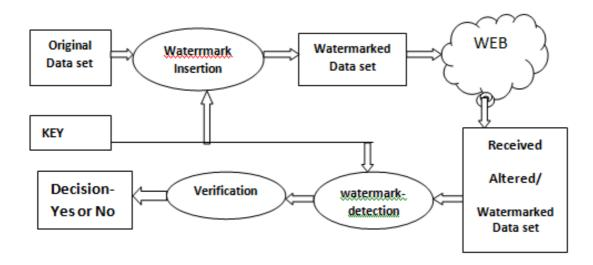
Fig1: Digital watermarking scheme
