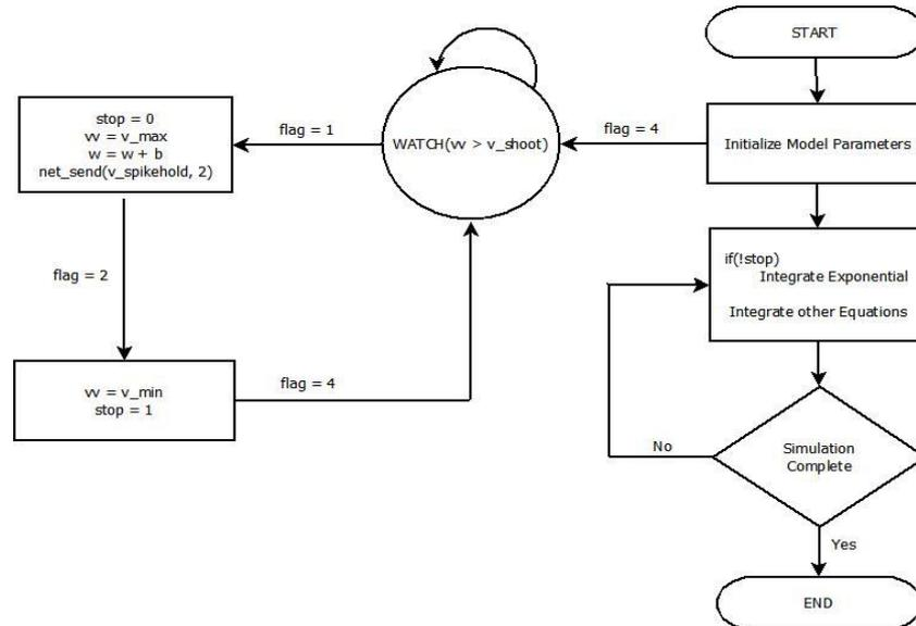
**Fig. 2:** V-I characteristics at AIS (left) and AdEx model implemented in NEURON (right).
