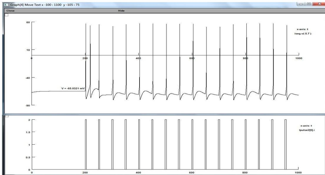
**Fig. 3:** Voltage response of the reference model to a series of regularly spaced current pulses.
