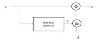
Fig. The un-sharp masking structure.
