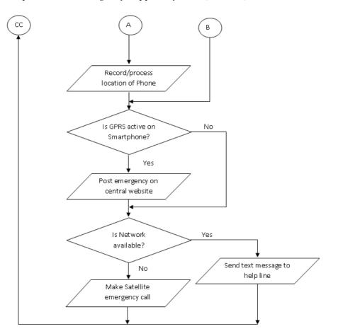
Figure 2. Flowchart of Smartphone-Based Accident Detection System
