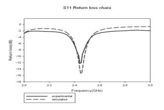
Fig3:Return loss chara with CSRR in Fig2(a),  $f_R = 2.45 GHz$ (Sigma plot<sup>TM</sup>)
