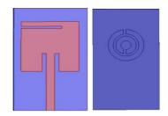
Fig1:(a) Substrate dimension:  $26 \times 45 \times 1.6$ mm.Patch dimension: $20.4 \times 21.7$ mm.Feed:  $25.06 \times 3$ mm. Slot:  $13.6 \times 1$ mm. (b)CSRR dimensions: $7 \times 1$ mm and  $4 \times 1$ mm rings. (HFSSv14.0)
