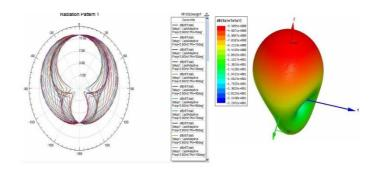
Fig6: 2D & 3D simulated radiation patterns(for all angles) of model in Fig2(b)
