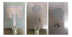
Fig5: Fabricated antenna models
