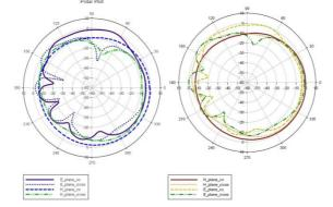
Fig7: Radiation patterns of E and H planes co and cross polarized components (a) antenna with 2 CSRR rings, (b) antenna with 3 CSRR rings(experimental)
