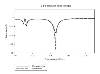
Fig4:Return loss chara with CSRR in Fig2(b),  $f_R = 2.45 GHz$ (Sigma plot<sup>TM</sup>)
