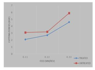
It was found that the cutting force of the treated tool decreased by an amount of 23% in comparison with the untreated tool.
