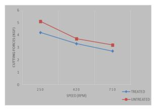
It was found that the cutting force of the treated tool decreased by an amount of 15% in comparison with the untreated tool.
