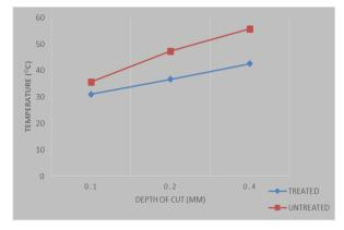
It was found that the tool tip temperature decreased by an amount of 20% in comparison with the untreated tool.
