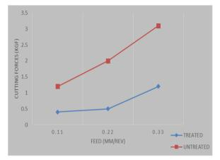
It was found that the cutting force of the treated tool decreased by an amount of 67% in comparison with the untreated tool.
