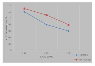
It was found that the cutting force of the treated tool decreased by an amount of 20% in comparison with the untreated tool.
