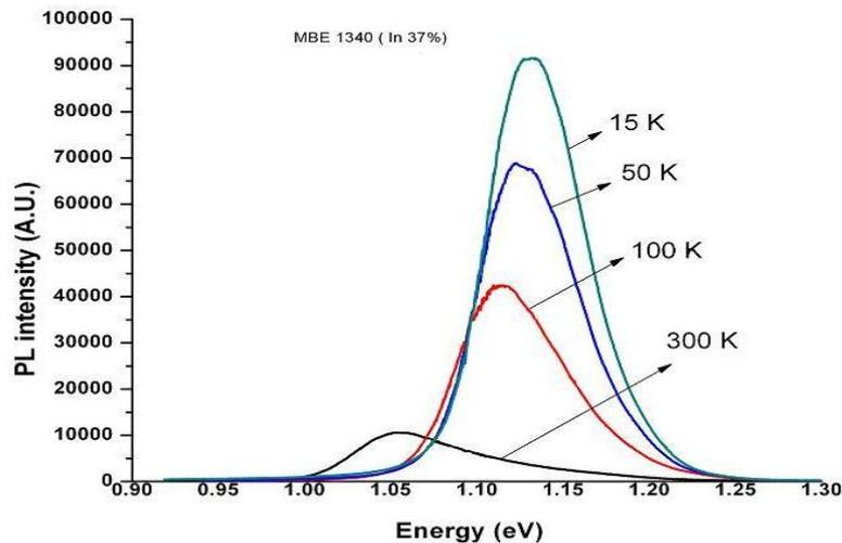
The temperature dependent PL spectra for InGaAs QWs
