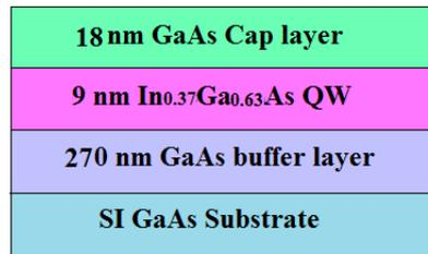
Fig. 1: The schematic structure of the sample.
