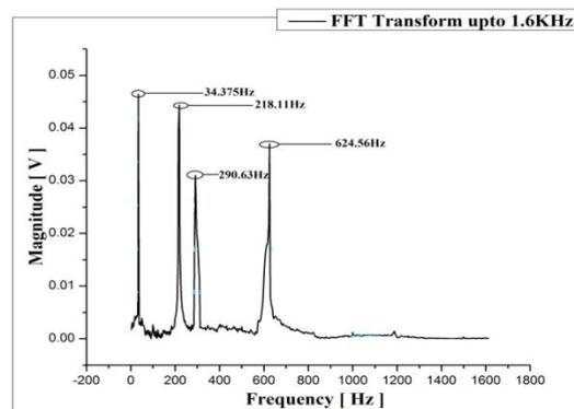
**Graph 6: FFT plot for 1 mm crack depth**
