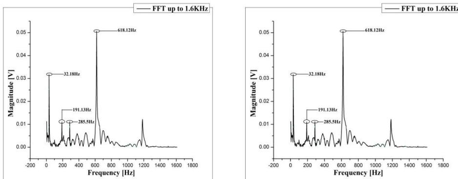
**Graph 7: FFT plot for 2 mm crack depth**
