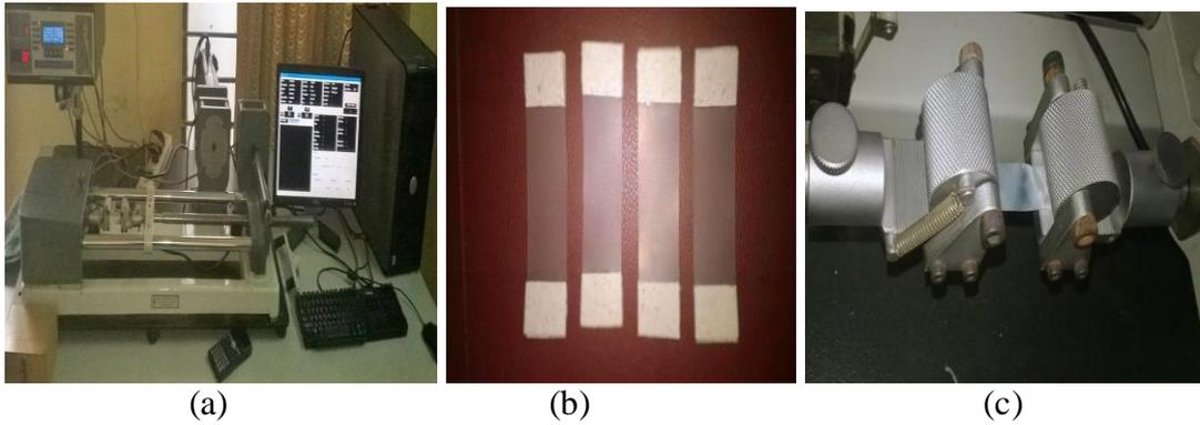
**Fig1: (a) Electronic tensometer (b) Prepared film test samples (c) Samples held under roller chucks**
