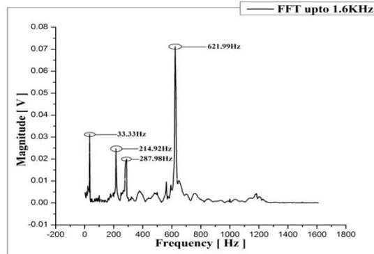
**Graph 6: FFT plot for 1.5 mm crack depth**
