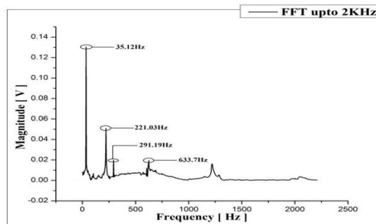
**Graph 5: FFT plot for 0.5 mm crack depth**
