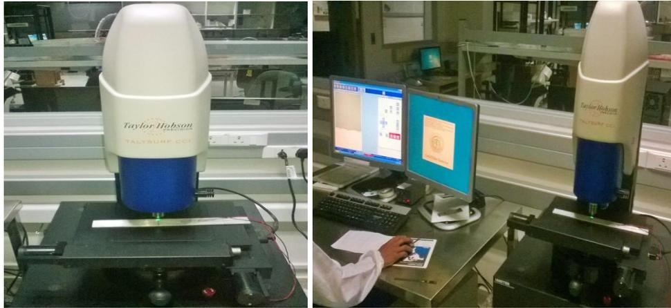
**Fig. 2: Taylor Hobson Talysurf 3D HD microscope to measure and achieve accurate crack size and depth: (a) optical microscope (b) machine setup**
