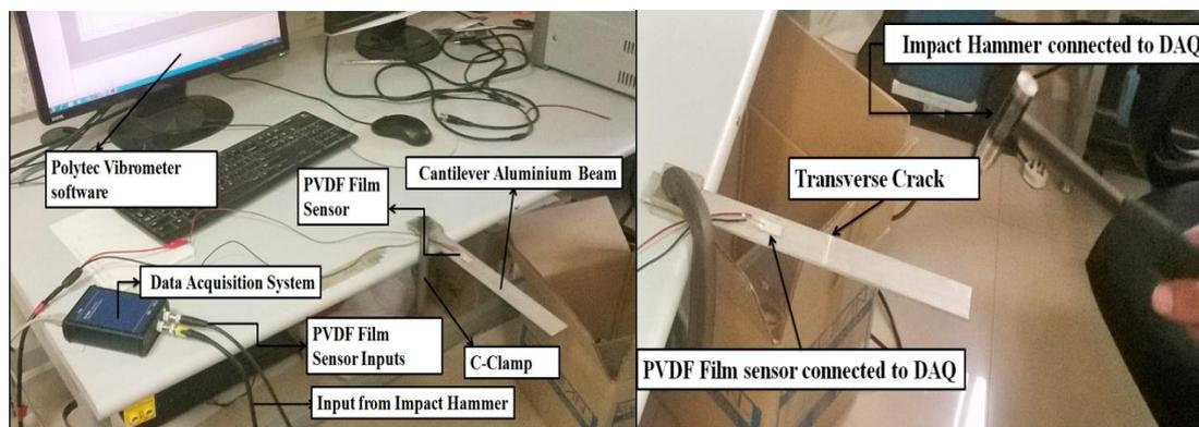
**Fig. 3: Experimental setup for crack and its depth estimation**
