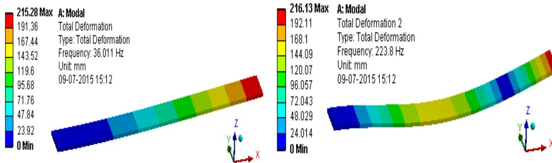
**Fig. 6: Mode shapes with frequencies for an intact cantilever beam**
