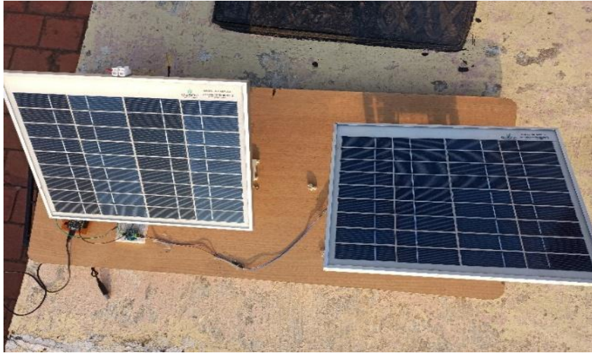
Fig. 12: Solar tracker power comparison with stationary solar panel
