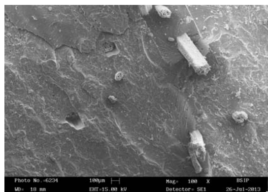
FIGURE 10(c): SEM image of Hybridized (5%) LGF/OMMT/UPR Hybrid NanoComposites
