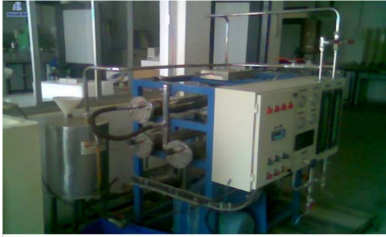
Fig 1: Experimental Set up for Ultra filtration and Nanofiltration Process
