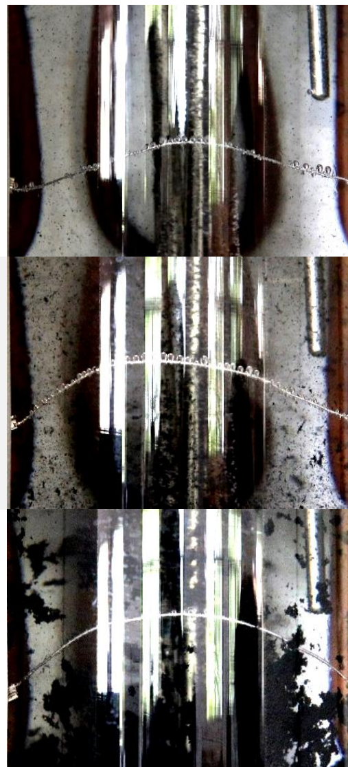
Figure.3.10(g,h,i) Video snapshots and analysis of bubbles using image-J image processing software during Nucleate pool boiling 0.1,0.2 and 0.4 wt.(%) at 0.1% vol.conc. of Graphene-MWCNT/Distilled water.
