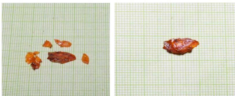
**Fig .1** Laboratory grown crystals of 1-2( 2,4-dichlorophenyl -3-(4-Dimethyl amino-phenyl) propenone(DDAP)
