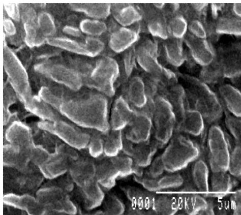
**Figure 5:** SEM image of ZnS nanoparticles.
