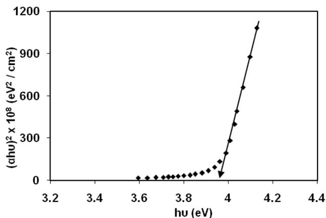
**Figure 3:** Band gap determination of ZnS nanoparticles.
