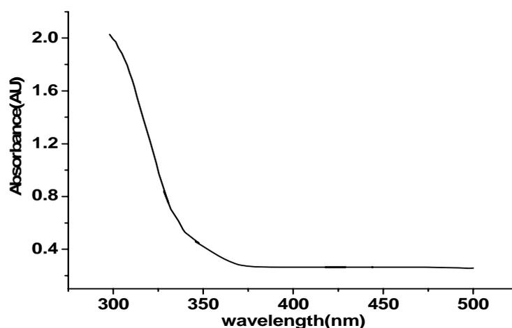
**Figure 2:** Absorption spectra of ZnS nanoparticles.
