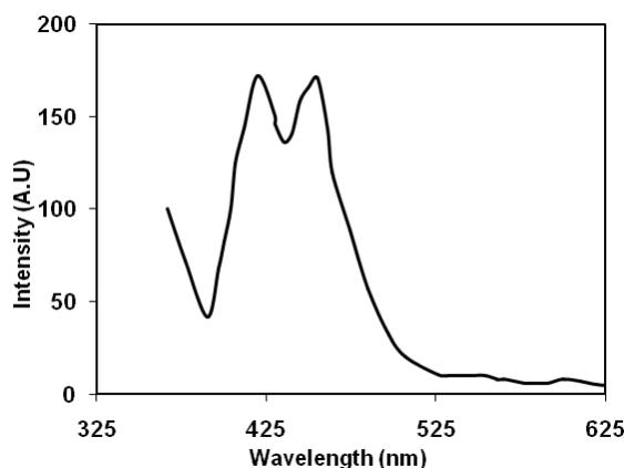
**Figure 4:** PL spectra of ZnS nanoparticles.
