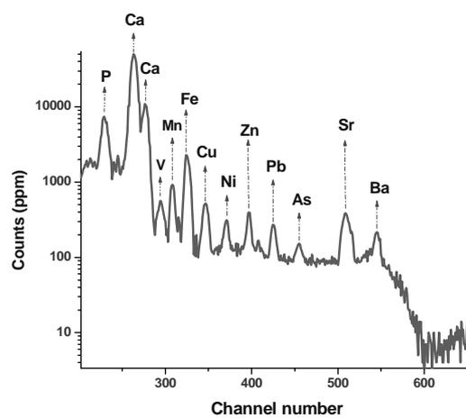
**Fig.3.** The external PIXE spectrum of dentine region of human teeth
