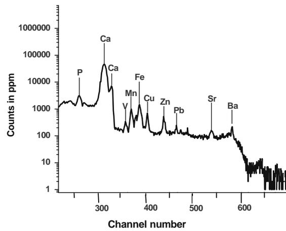
**Fig.2.** The external beam PIXE spectrum of cementum part of human teeth
