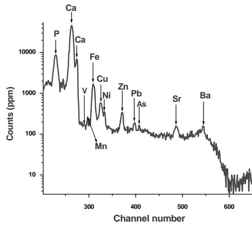
**Fig.1.** The spectrum of dental enamel of human teeth obtained from external PIXE
