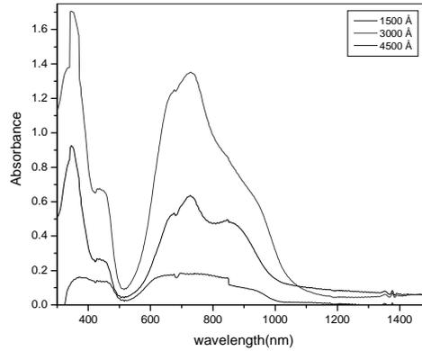
**Figure 4:** Variation of absorbance with wavelength of PbPc films for different thicknesses.
