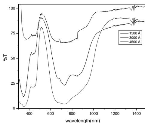
**Figure 3:** Variation of transmittance with wavelength of PbPc films for different thicknesses.
