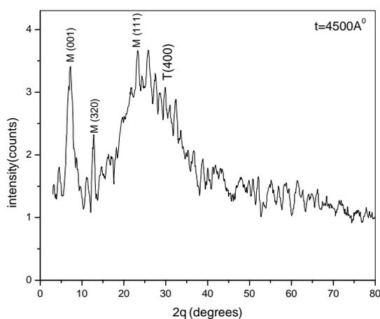
**Figure 1:** XRD Patterns of PbPc Films for thicknesses 450 nm.
