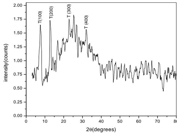
**Figure 2:** XRD Patterns of PbPc Films for thickness 450 nm at 373 K temperature.
