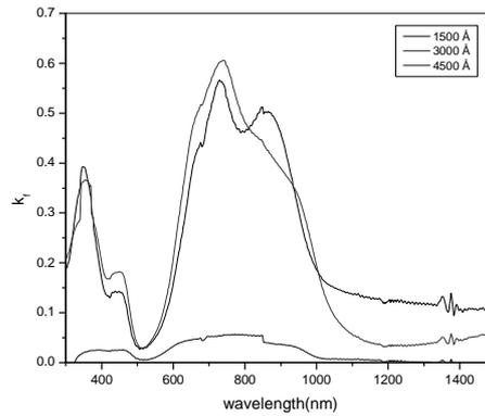
**Figure 5:** Variation of extinction coefficient ( $k_f$ ) with wavelength of PbPc films for different thicknesses.
