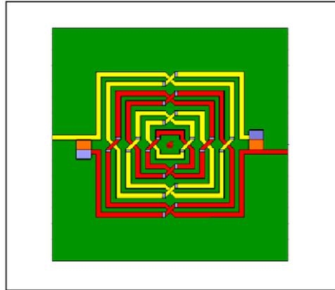
**Fig.2.** Differential Transformer based BPF
