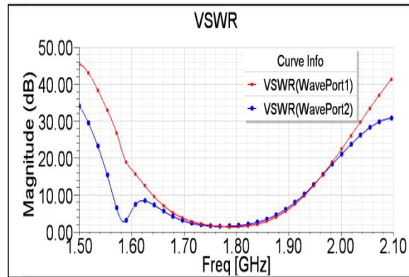
**Fig.5.** Variation of VSWR with Frequency [GHz]
