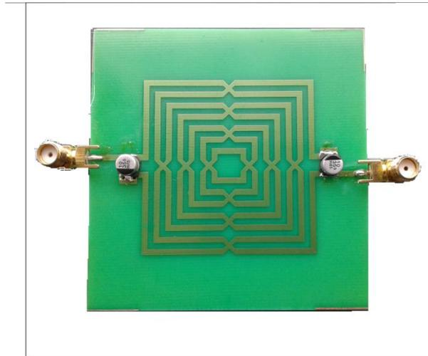
**Fig.6.** Image of fabricated BPF
