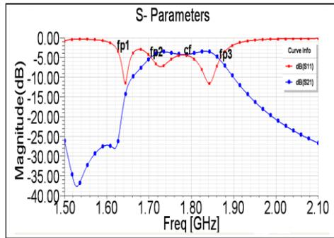
**Fig.3.** Variation of S-parameter with Frequency [GHz] (initial design)
