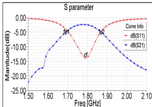
**Fig.4.** Variation of S-parameter with Frequency [GHz] (modified design)
