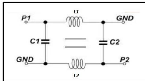
**Fig.1.** Equivalent diagram of BPF
