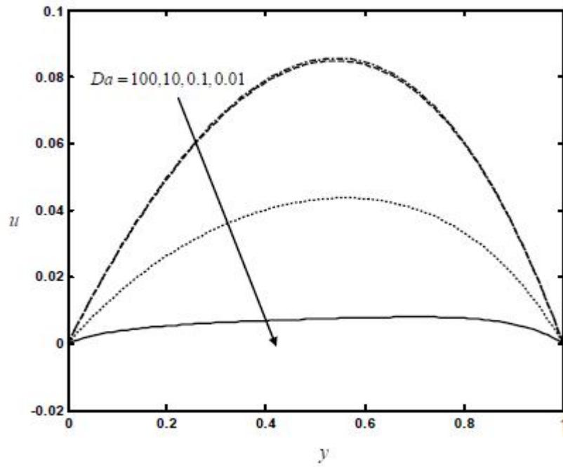
**Fig. 3.** Effect of Darcy number  $Da$  on  $u$  for  $Gr = 1$ ,  $We = 0.2$ ,  $M = 1$ ,  $r_T = 0.5$  and  $Re = 1$ .
