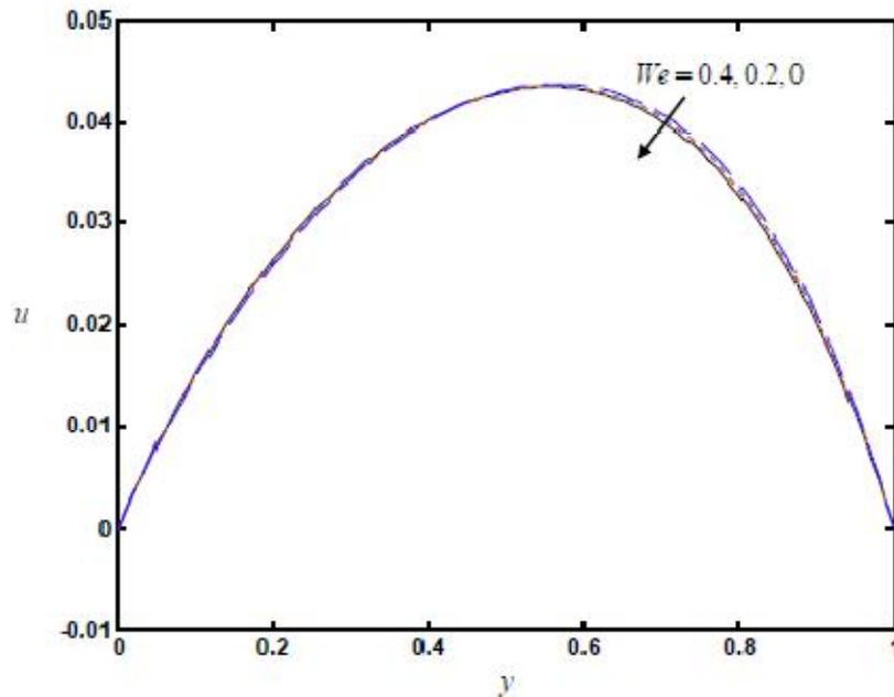
**Fig. 2.** Effect of Weissenberg number  $We$  on  $u$  for  $Gr = 1, Da = 0.1, M = 1, r_T = 0.5$  and  $Re = 1$ .
